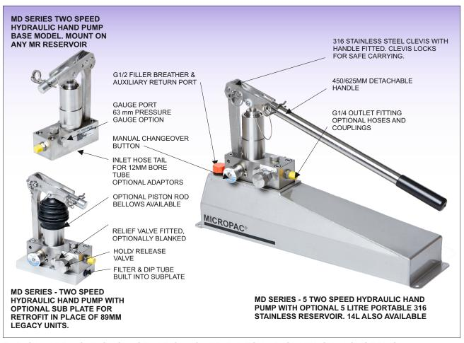
TYPICAL APPLICATIONS: ACTUATION, OVER-RIDES AND SHUTDOWN SYSTEMS, PRESSURE TESTING, FILLING AND CHARGING TO 1000 BAR MULTI FLUID USE ON "SKYDROL" AND OTHER SPECIALIST MEDIA. COMPACT STAINLESS PUMP TO REPLACE LEGACY ALLOY 2 SPEED UNITS
