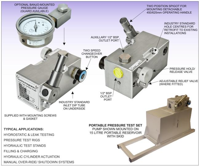
A rugged reliable two speed manual changeover hand pump 6 models up to 1000 bar • low corrosion • industry standard retrofit • reservoir available
