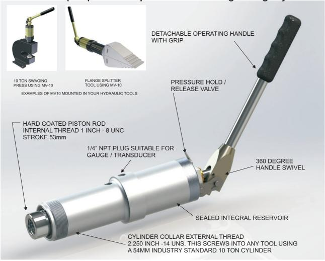
TYPICAL APPLICATIONS: LOAD HOLDING, JACKING AND WORK HOLDING. DESIGNED FOR HYDRAULIC TOOLS WHEN FITTED INTO YOUR OEM OR CUSTOM DESIGN. RAM + HOSE + 2 SPEED PUMP IN ONE UNIT.
